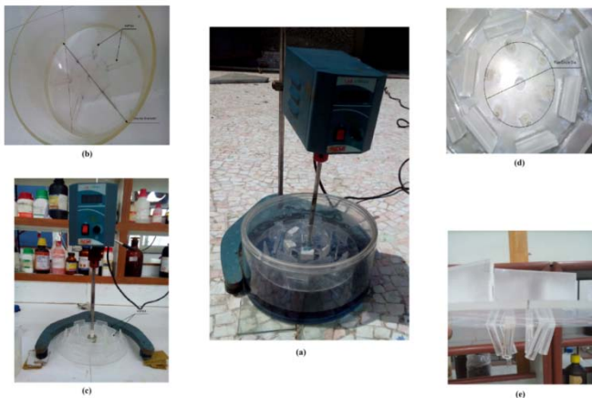
Fig. 2: (a) Reactor, (b) Baffles configuration, (c) Vanes configuration above the plate, (d) Pipe circle diameter, (e) Pipes for water recirculation
